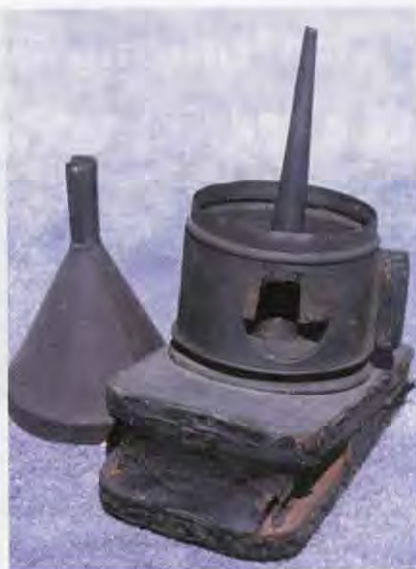
The internal construction of the Simplicity Cold Blast Smoker. Look at that slender blast tube! Have you ever seen anything like that inside a smoker?
