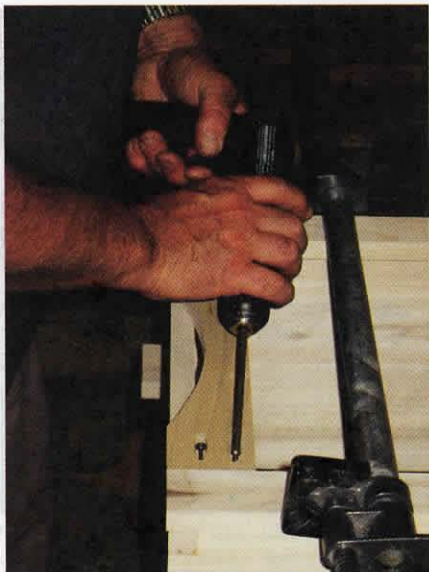
Attaching face frame rails and stiles with pocket screws.
