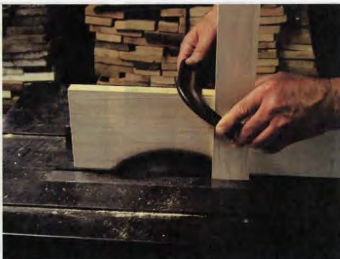
Cutting door mortise.
