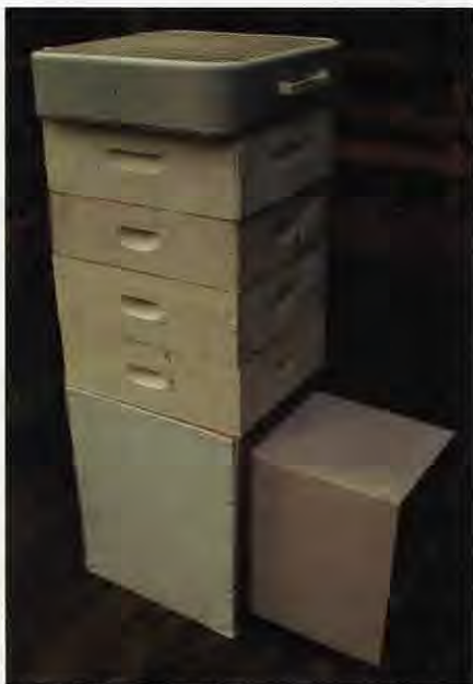
A simple rig for drying honey in the supers. Note that the dehumidifier faces into the box at the bottom while the box fan lies on top of the supers to pull air through the stack.
