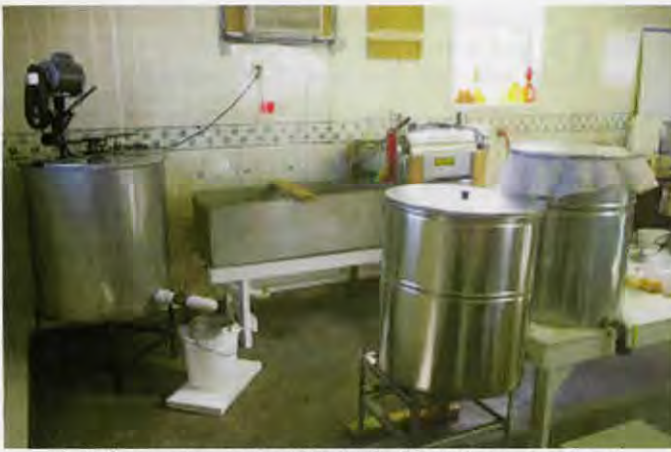
Radial extractor, uncapping tank, Maxant uncapper and bottling tanks.
