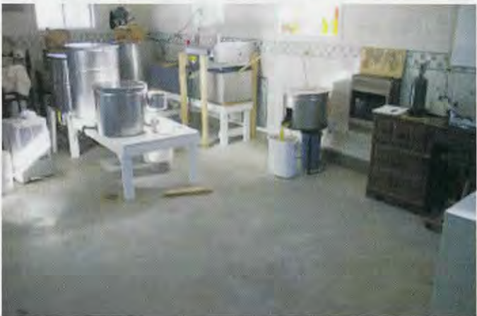
Bottling tanks on the left, extractor, tray and uncapper in the corner.
