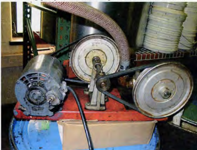
A honey pump with a reversing 1/2 H.P. electric motor.
