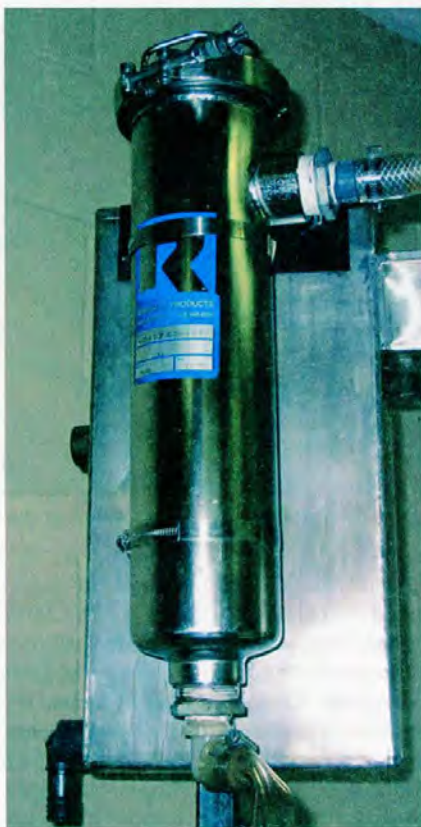
The inline filter. Pressure should not exceed 40 psi. To clean, release pressure, remove cap, filter and wash inside or replace.
