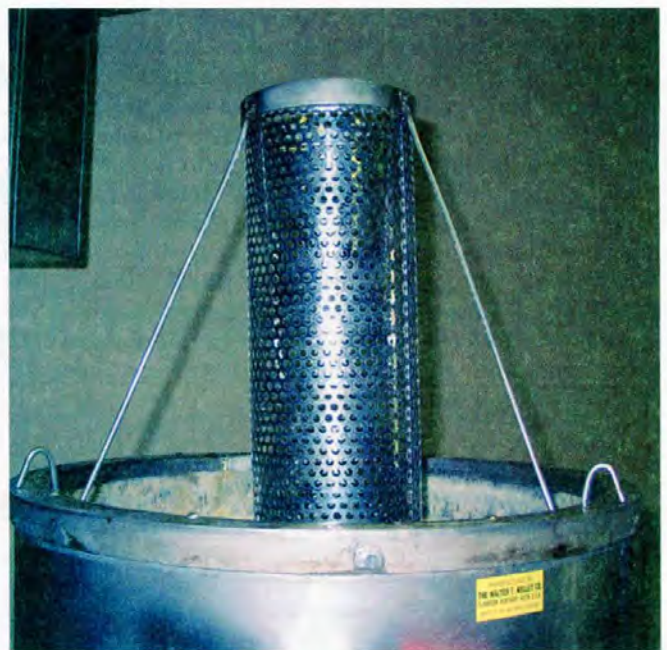
A gravity strainer above a bottling tank, supported by a tripod system.
