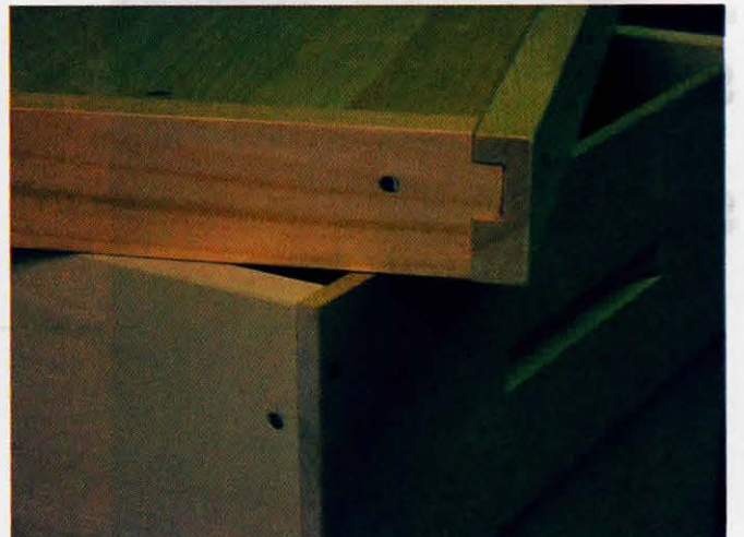
Bottom Board Joint close up.
