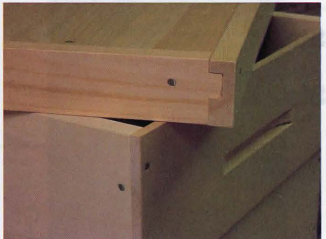
Bottom Board Joint close up.
