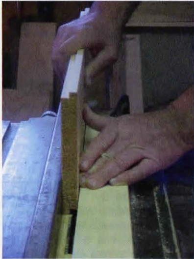
Bottom Board Step 2 - Cutting shiplaps.
