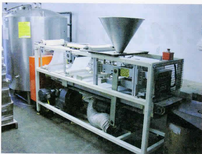
BeePro patties come together in this machine where raw materials are blended, mixed, formed, sheeted and boxed.
