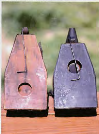
Figure 2. Moving the valve on the bellows. On the left, the valve is near the back end of the smoker away from the blast tube. On the right, the valve is moved toward the front of the smoker. Note also the springs on the outside of the bellows, as was typical of early Clark smokers.
