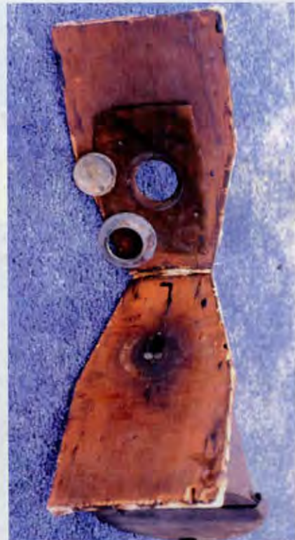
Figure 5. The parts of the cleaning cap disassembled and seen from the inside of the bellows. The threaded piece of metal would be flipped over and inserted in the hole in the board. The original fabric of the bellows had deteriorated away and unexpectedly revealed the inner workings of a virtually unknown smoker design.
