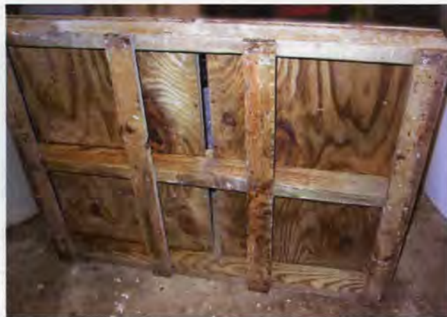
The bottom of the pallet showing four brace boards and the center drain hole.
