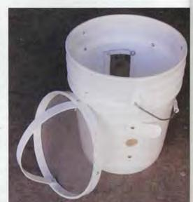
Screen cover on outside. Ring #two positioned inside pail. Hole for vacuum hose with hole cover in place.
