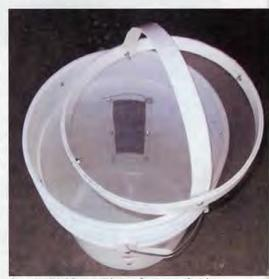
Screen Divider – Ring #four on the inside, ring #one on the outside. Screen in between four and one. Ring #three as handle.
