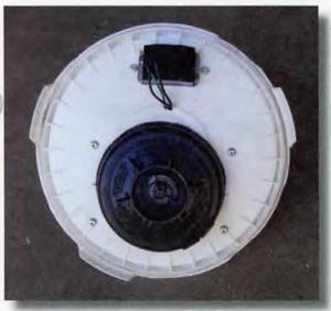
Inside the lid, with modified tabs and motor and switch held in place.
