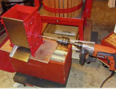
Scratter, which chops the whole apples into little bits, run with a drill that has a lockable trigger is much faster than the handwheel. Next upgrade an electric motor and pulleys.
