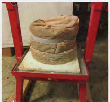
Winepress can be used as either a cloth and rack press or as a basket press with spacer plates to make it more efficient like a rack press. Wine press with apple scratter converted to a rack and press setup or with spacers used in press basket to make it much more effective than just pressing a single big bag (basket removed to see configuration of spacers and bag).
