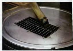
Honey drains from our 50-frame extractor into the sump and is pumped into settling tanks.
