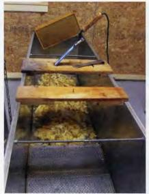
This extra large uncapping, holding tank will contain several days cappings which drain through a screen, reducing the amount of honey going into the wax melter.
