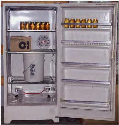
near the bottom. And, finally, he installed two plug-in fixtures in the outlets. Incandescent light bulbs of various sizes are plugged in when needed to heat the inside of the unit.
