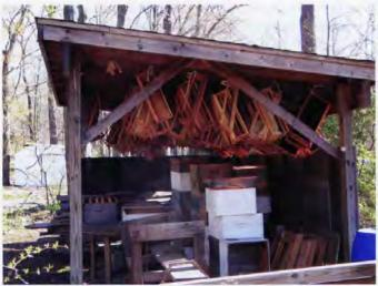
This open structure found on the grounds of the Pfeiffer Center for Biodynamic agriculture in New York state makes use of sun light and ventilation to allow empty unused frames of comb to be stored year-round without damage from wax moths or mice.
