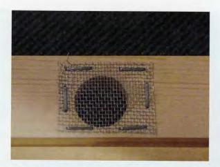
**Step 4:** Drill 1" vent holes in the sides (parts 2). After drilling the holes, staple window screen to the inside to prevent the bees from escaping.
