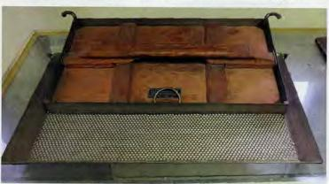
Foundation mold with lid placed back halfway.
