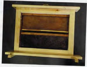
**Step 15:** Mount the glass in the door using silicone seal and let it dry. The glass and silicone will hold the door frame rigid.
