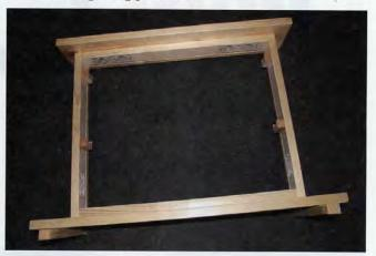
**Step 10:** Cut the stabilizing legs (parts 6) and attach them to the bottom of the unit. Do not cover any screws you have used so far. You may want to disassemble the unit in the future without removing the legs.
