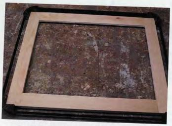
**Step 13:** Glue the door frame together. Make sure the joints are tight and the door is square.
