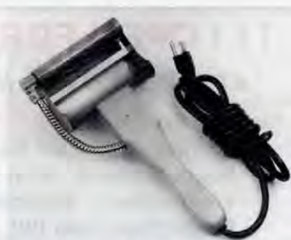
The uncapping plane. The blade is heated, and moved down the surface of the comb, with cappings falling below.
