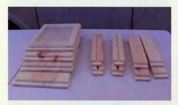
2. To make the window in one side of the bee box, cut 1" strip from the top and bottom of one 113/4" piece. From the center strip, cut a 13/4" piece from the rebated end and a 1" piece from the opposite end. Now make a 5/16" deep saw cut in the edge of the four pieces to receive the plastic glazing window. Then from the remaining material, cut four 2" x 2" triangular feet.
