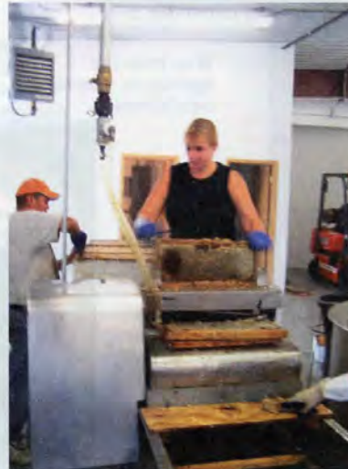
Loading one of the Bogenschutz uncappers. Frames are scratched if not uncapped, and top and sides cleaned before going into the extractor.
