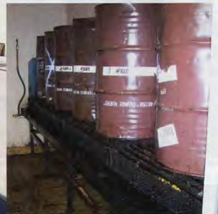
Machine (left) that grasps a wax barrel and turns it upside down to place it on the wax-melting table, so it rests on hot pipes.
