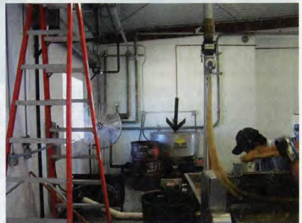
Piping honey from the extractors to the wax spinner (arrow).
