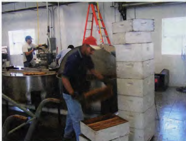
Unloading extractor. Boxes are moved out on a hand cart.
