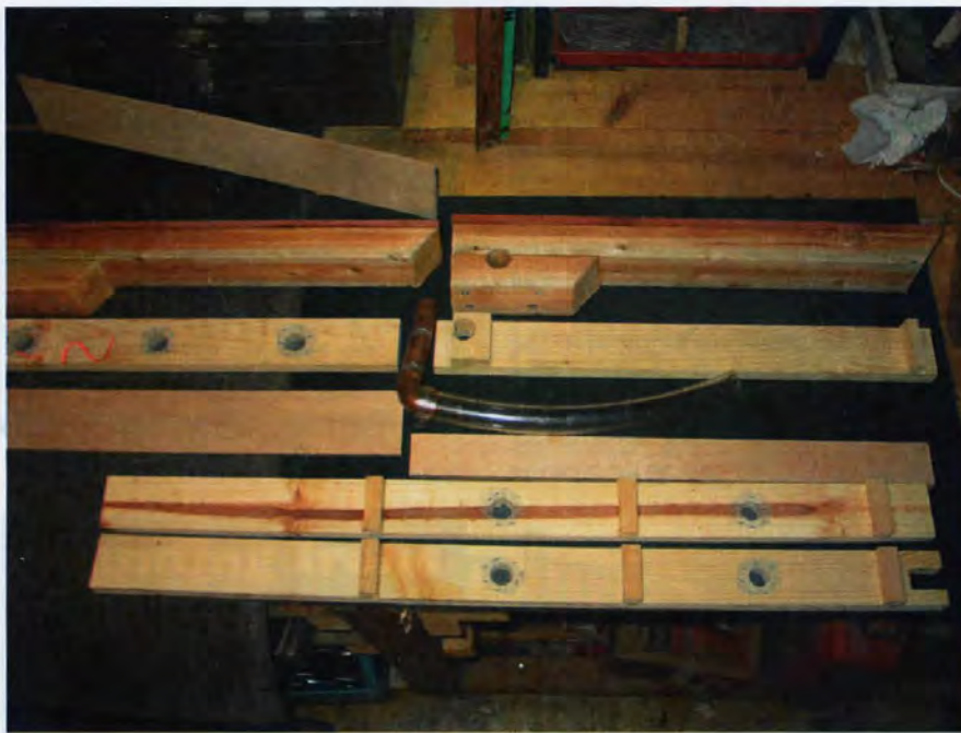
L,R sides with screens; top and bottom; upper and lower wall mounts; entrance pivot copper and vinyl tube, cleanout slide.
