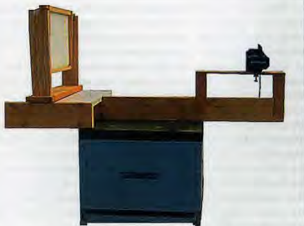
Stand for holding the digital camera and hive frame, placed on top of a super.
