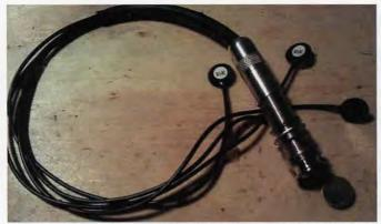
K&K Pure Classic (four-head piezo-ceramic transducer with endpin jack). I cut off the connector and installed each in a single frame.
