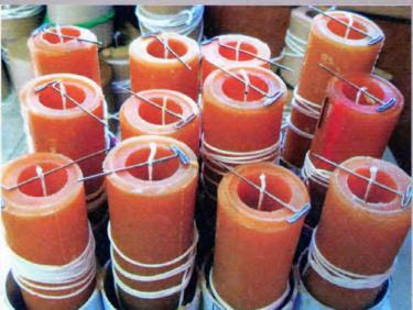
Our molded candles are made by securing wick, at the mold opening, with a sewing pin, pulling it tight and wrapping extra wick around mold to make it self-threading. Molds are placed in PVC tubes set in wooden frames and placed in a shallow container.
