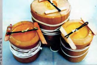
Poly molds are our choice for making novelty candles. Note that extra wick is wrapped around mold so that they are restrung as candle is removed.
