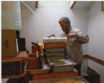
Kirk Webster makes 2-3,000 sheets of foundation every year with his hand-cranked mill. The tube above feeds water into a homemade cylinder that drips onto the rollers, keeping them cool. (photo by Dean Stiglitz)
