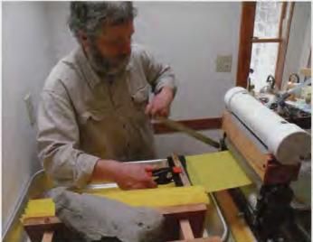
A snowy Vermont day in a room warmed up for wax foundation making. As Kirk Webster cranks the mill, he pulls the embossed foundation sheet with a wood and plastic grip that is attached to a clamp. (photo by Dean Stiglitz)
