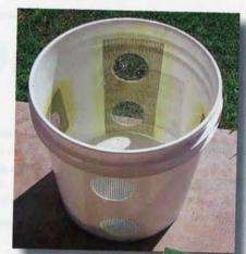
9. If you use the vacuum often, you can also attach the screen to the inside of the bucket by using Epoxy glue. The Epoxy comes in all types and applications, so be sure and use one that will work with metal and plastic.
