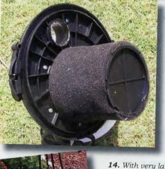
14. With very large swarms or cutouts. or very high outside temperature, we will empty the vacuum into a holding bucket. This helps in reducing the mortality rate. We just placed a top bucket onto a bottom bucket and cut areas out for ventilation. Notice the #8 screen taped onto the outside.
