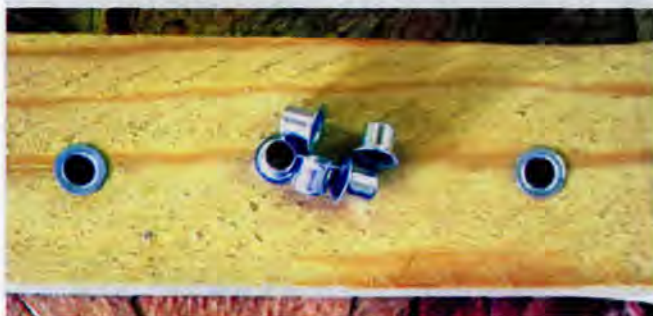
Two eyelets installed in an end bar.
