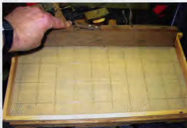
An electric wire embedder melting support wires into the foundation.
