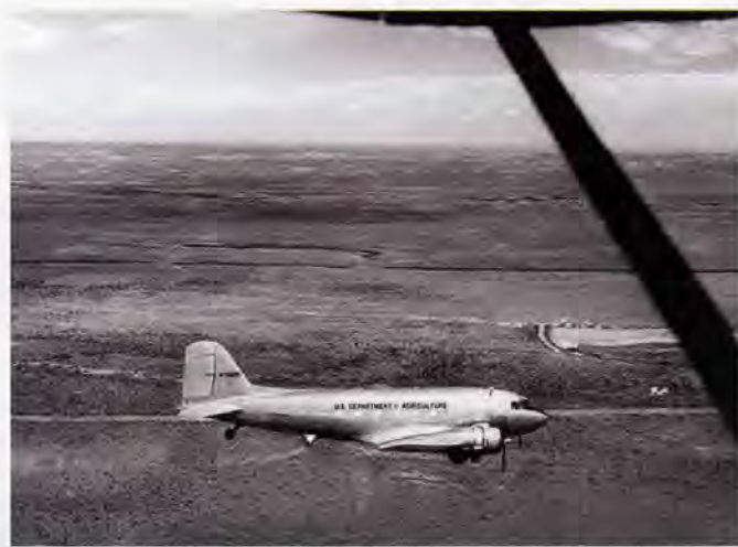
Flying from 100 to 300 feet above grasshopper-infested rangelands in Johnson County, WY the C-47 (DC-3) spreads bait at the rate of 300 pounds a minute in June 1949. Its two three-man crews make it possible to cover 20,000 acres in a 14-hour day, with each acre receiving five to 10 pounds of bait. Photo courtesy of National Archives and Records Administration.
