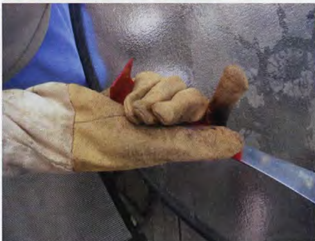
The plastic coated canvas gloves are a bit less bulky, but finger length can be an issue.
