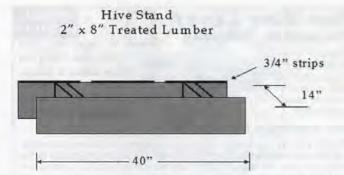
the hive stand design that has been used at Cornell University I used 2 x 8" treated lumber By installing a 34" strip on the back of the hive stand, I gave the hives a slight lean to the front.
