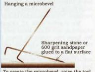
To create the microbevel, raise the tool 3-5° above the primary bevel
