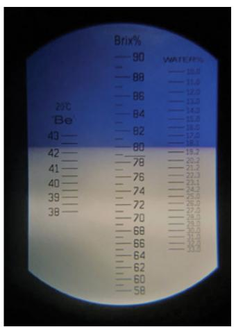
This is what you can see when you look into the eyepiece of a honey refractometer. The honey measured here has a moisture content of approximately 18.5%
