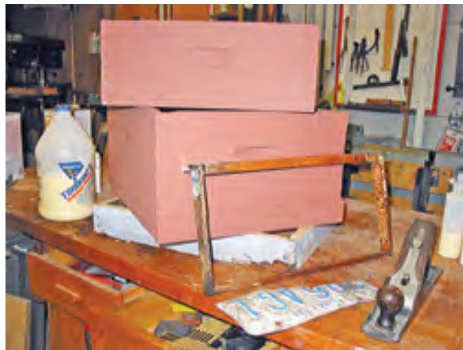
Repaired equipment. Note the top deep hive body that was cut down to a super. The equipment is stacked on the white cut-off. Note the upper repaired right corner on the deep and the bottom repair strip. The frame has a repaired top bar lug. Paint makes the repairs look even better.
