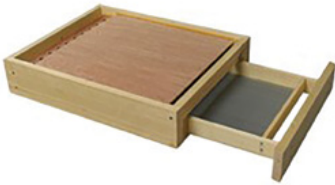
Sundance Bottom-Mount Pollen Trap (photo courtesy: Betterbee). The bottom mount is the original type trap and works very well. Bottom-mounted traps are placed between the bottom board and the brood chamber. The bees are forced to go through the trap to get into the hive. The pollen trap has a grid, like hardware cloth, to scrape pollen off the bees' hind legs as they enter the hive. Often there is an option to allow the bees to get into the hive without going through the trap if you do not want to collect pollen but leave the trap on the hive. The pollen-collecting drawer is typically accessible from the hive's rear. The pollen traps are usually sold assembled. Drone escapes are placed in the pollen trap opposite of the drawer.
