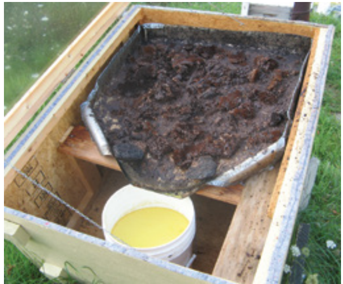
This solar wax melter utilized a double pane replacement glass window for the lid. Built for maximum efficiency, it will melt wax on sunny days when daytime temperatures never get over 60°F (16°C).
