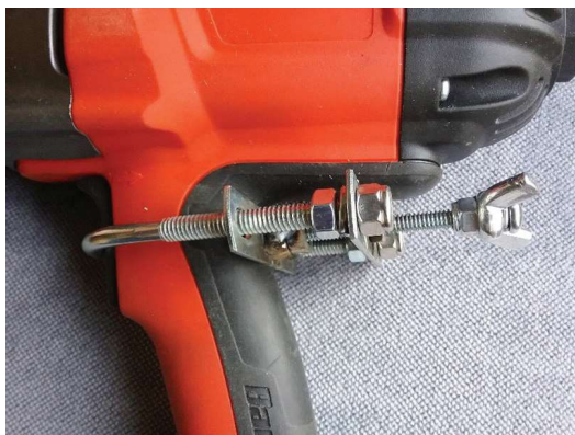
Note: The nuts welded to the sliding plate are not attached to the adjusting bolt. They are used to keep the adjusting bolt point in position on the sliding plate.
