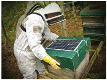
Solar cells recharge the batteries in the ApisProtect sensor unit.
