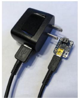
**Figure 4.** OEI's WiFi Hive Scale comes with a battery charger which can be plugged in via a standard mini-USB cable.
