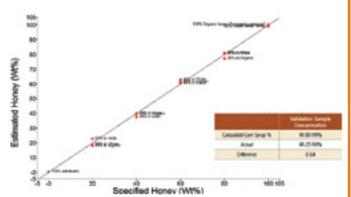
**Figure 2.** PLS model of multiple honey types adulterated with corn syrup. The table inset shows the results of a validation sample
