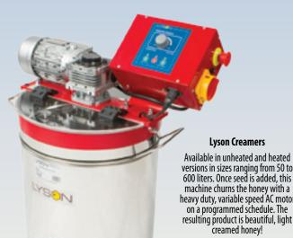
Available in unheated and heated versions in sizes ranging from 50 to 600 liters. Once seed is added, this machine churns the honey with a heavy duty, variable speed AC motor on a programmed schedule. The
