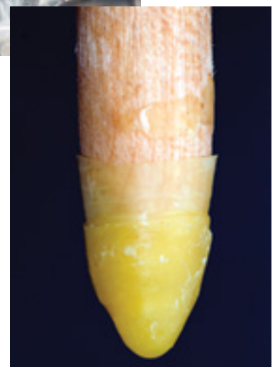
Finished wax cup ready for twisting off the dipping rod.
