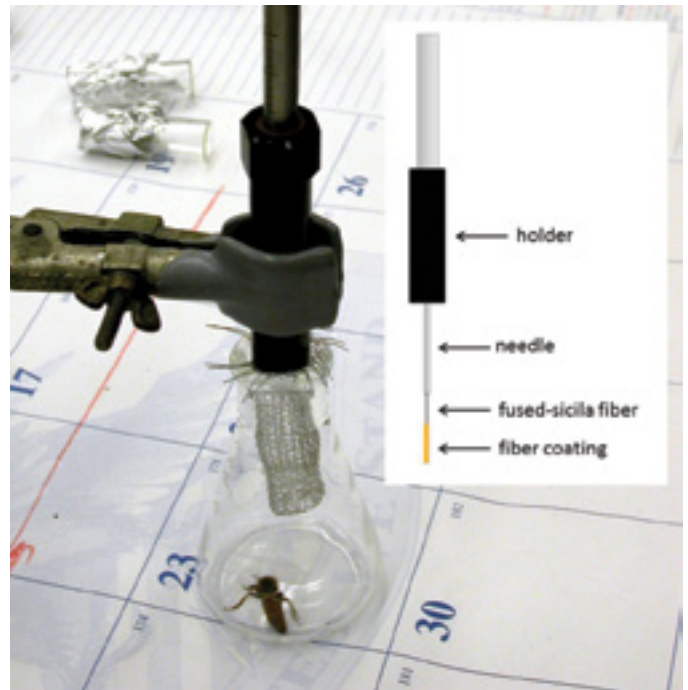
Figure 1. A live queen, in flask, is sampled for volatile compound emissions using a SPME fiber. The fiber is protected by a wire-mesh guard during sampling. Inset: diagram of a SPME fiber.
