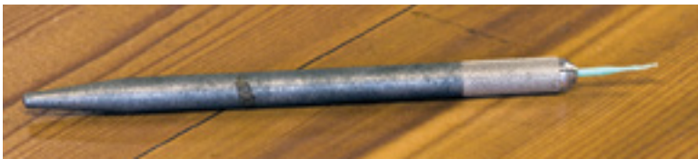
A modified plastic toothpick in an X-Acto handle.
