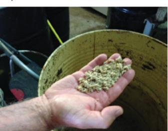
Wax flakes out of the separator.
