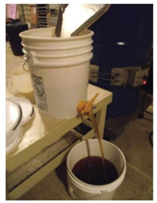
**Problem** #8 – solved – To bridge this gap I built a chute made of  $\frac{3}{4}$ " wood covered with aluminum. The sides are turned up to keep the honey in the chute and
