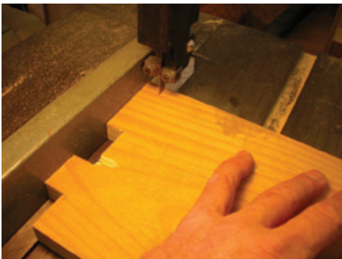
With the band saw fence set to a 3/4" cut, remove the wood to reveal the fingers.
