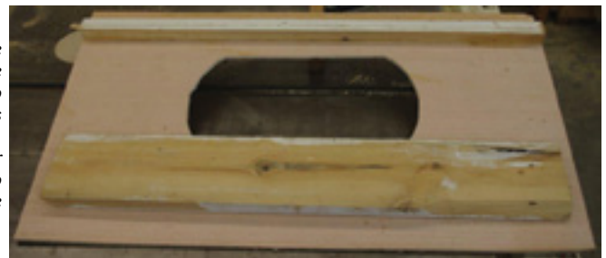
Photo shows the bottom of the template used to create handholds on the super sides. Place template over side, center, clamp to work place and route away.
