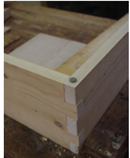
Drive the nail home to assure the drill bit is not too large or too small. The nail should need a medium tap from the hammer but not split the wood as it is driven.
