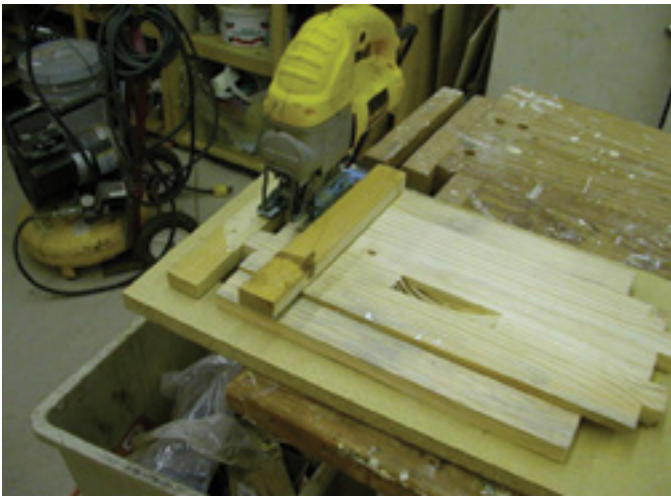
Some scrap pieces are easily assembled into a hold down, guide and stop. Note the hand holds chewed out with the dado set which lead to the router and template method of cutting hand holds.
