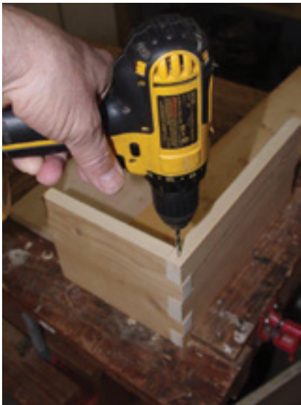
Clamp a piece in place and slide in its mate. Drill a pilot hole for the nail.
