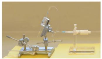
The Schley Instrument with a Harbo large capacity syringe. Fine precision is required, choose instrumentation carefully as there is no standardization and quality varies in equipment.
