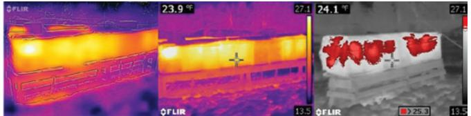
Wrapped hives at Ft. Missoula - FLIR. 1st Generation FLIR ONE with MSX technology (left), FLIR E60 professional camera (middle), FLIR E60 with grey/red (hot) thresholding set at 25.3°F. Stated resolution of the FLIR ONE 4,800; FLIR E60 72,800 radiometric pixels.
