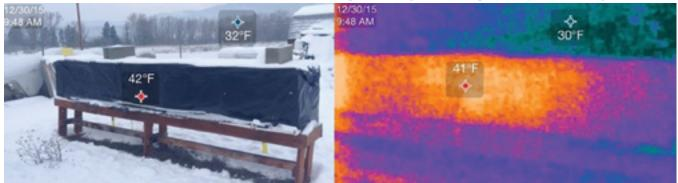
Wrapped hives at Ft. Missoula - SEEK THERMAL. Ipod digital camera image (left), SEEK THERMAL COMPACT IR image (right). Stated resolution of the Termal Compact is 32,136 radiometric pixels.
