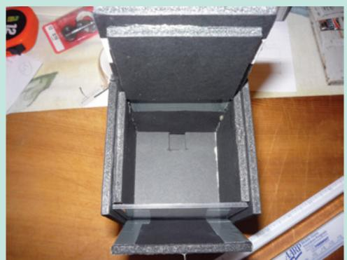
**Figure 3.** Interior view showing the sliding door, closed, between the catching compartment and the holding compartment.
