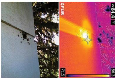
The panel contained insulation on the top, but was not insulated in the bottom as designed, which provided the cavity where these bees decided to make their home. Since this call, I've had chances to prove the thermal camera time and again as being a very valuable tool in finding and orienting hives for removal. I only wish I had the camera sooner.
