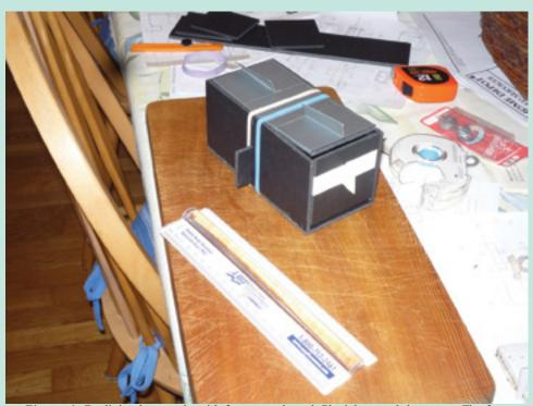
**Figure 1.** Beelining box made with foam core board, Plexiglas, and duct tape. The foam core board pieces are glued together. The Plexiglas top and its hinged covers are fastened with rubber bands. Hinges are duct tape.
