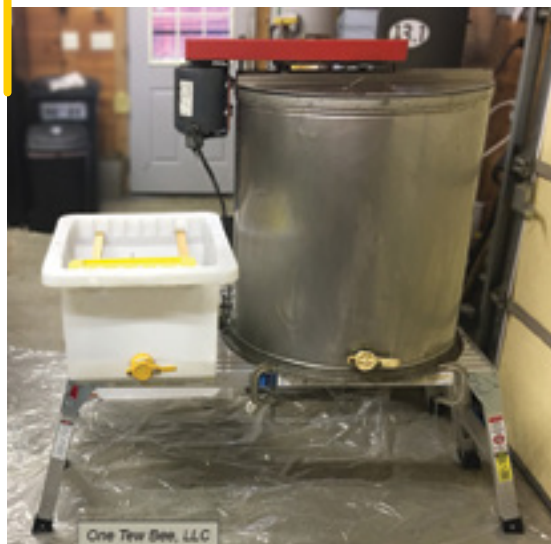
Figure 2. A collapsible work platform used as an extractor stand. Later, to provide a wider platform, another stand was added.
