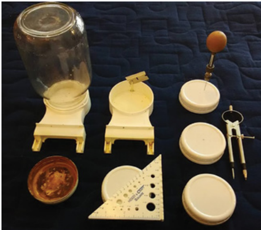
Left to right: Feeder jar with new cap above a rusted metal cap, Plastic jar holder showing where to cut out a rib above a hobby square and new cap, Pin vise with sewing needle to poke holes above a marked cap (layout marks are not visible) and compass above a completed cap (again holes are not visible in the picture)
