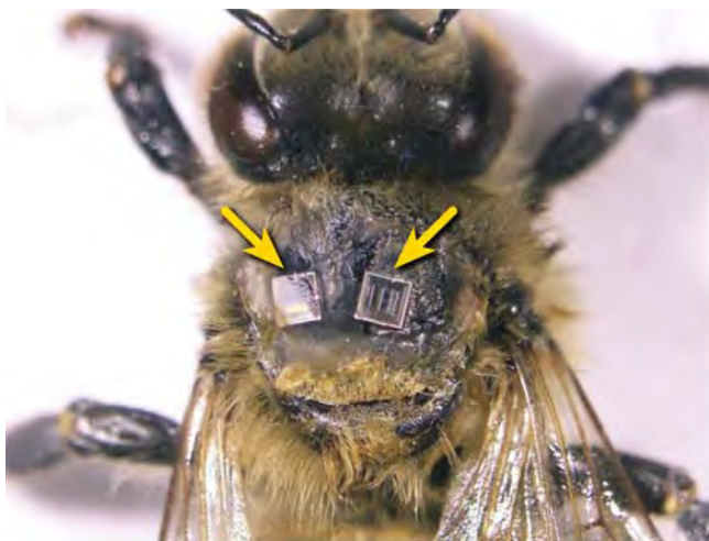
Automated behavioral monitoring of honey bees. Left Panel: Bee with two radiofrequency identification (RFID) tags. RFID readers placed at the hive entrance allow for automated monitoring of flight behavior (Tenczar and Lutz et al. 2014). Image from P. Tenczar. Right Panel: Bees with barcodes. Machine vision and machine learning allow for automated monitoring of in-hive behavior (Gernat et al. 2018). Image from B.M Jones and T. Comi.
